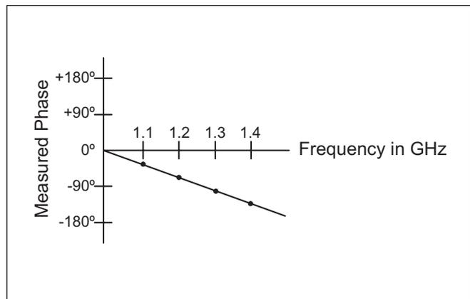
Figure 10. Electrical Delay
