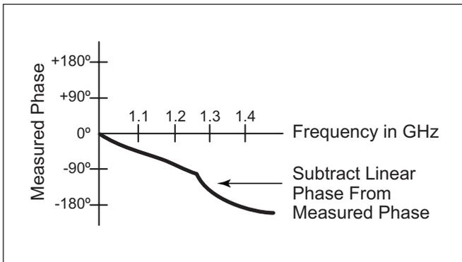
Figure 12. Phase Difference Increases Linearly with Frequency
