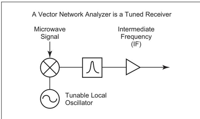
Figure 4. Network Analyzer is a Tuned Receiver
