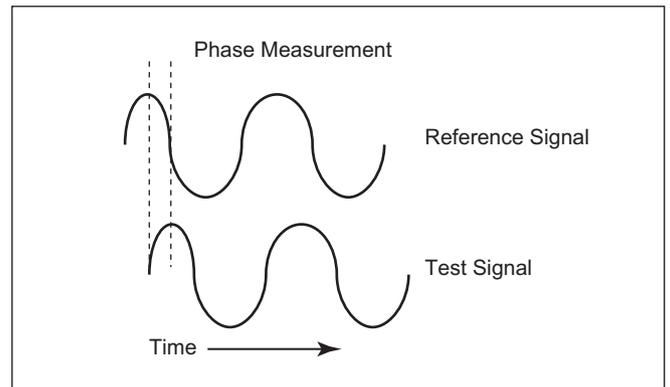
Figure 5. Signals with a 90 Degree Phase Difference
