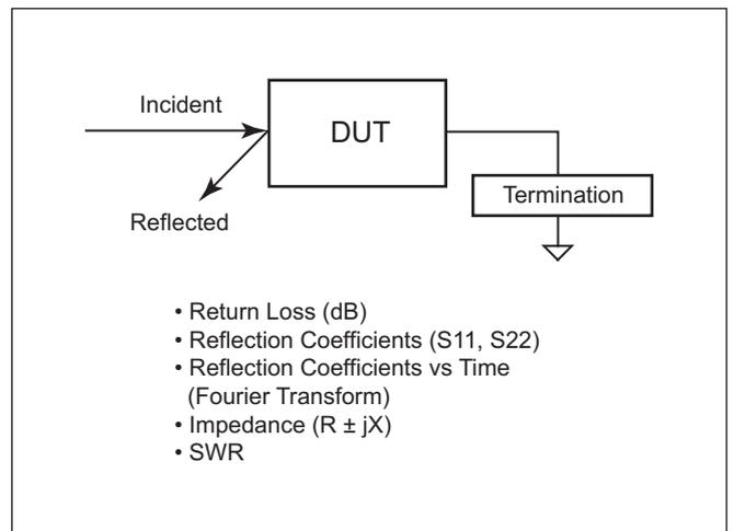
Figure 2. Reflection Measurements
