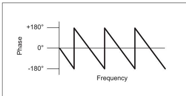
Figure 16. Linear Phase with frequency Waveform
