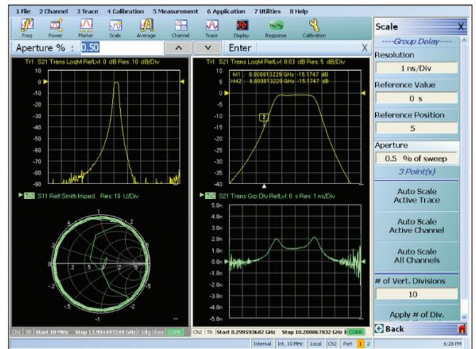
Figure 20. VectorStar Display of Group Delay measurement of a wireless communication filter
