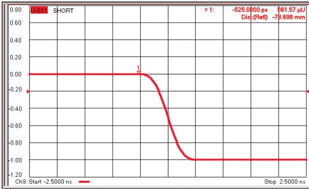
Figure 39. Low-pass step response of a short.
