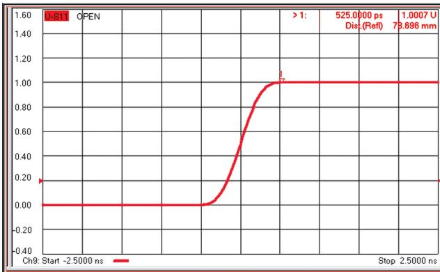
Figure 40. Low-pass step response of an open.
