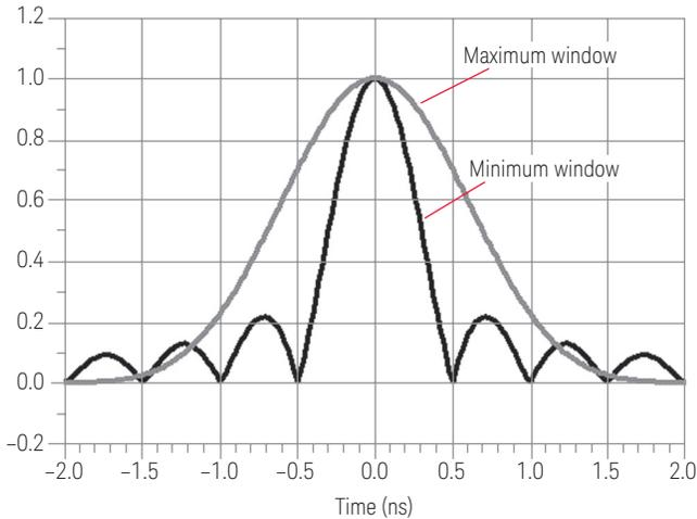
Figure 24. Comparing minimum window and maximum window.
