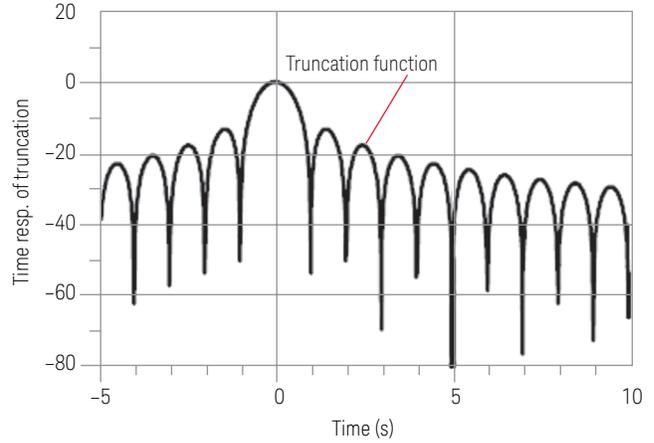
Figure 4b. Truncation causes ringing in time domain.
