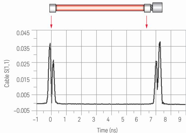
Figure 6b. Reflection responses of the same cable in time domain.
