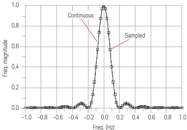
Figure 3a. Continuous function and discrete (sampled) function.
