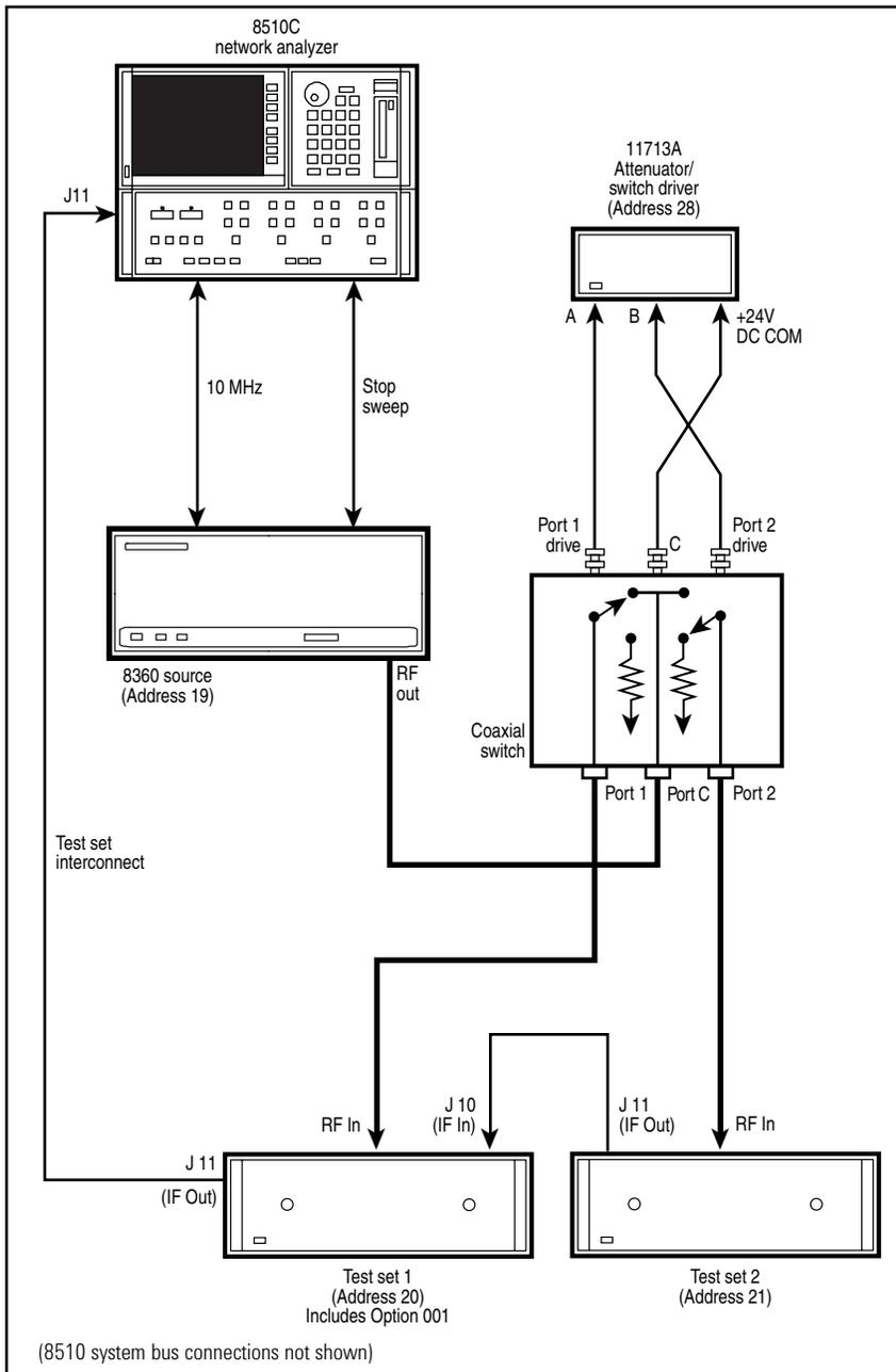
**Figure 2. Agilent 8510 dual coaxial test set configuration**
